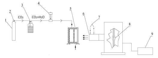
Fig. 1. Schematic illustration of the batch reactor system for the CO<sub>2</sub> photoreduction test: 1) cylinder of CO<sub>2</sub>; 2) gas cylinder valve; 3) water bubbler; 4) gas flow meter; 5) photoreactor equipped with a quartz window; 6) water filter; 7) inlet and outlet cooling water; 8) xenon lamp; 9) feeder
